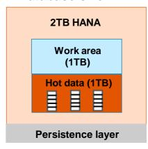
Expand HANA database capacity with warm data that is 2x the size of hot data
